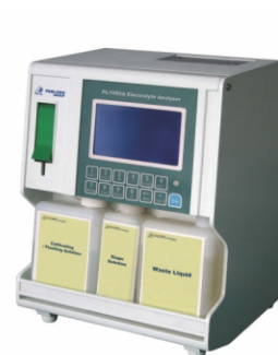
MK-PL1000A Electrolyte Analyzer Test Items: K + , Na + , Cl - , Ca ++ , PH Electrodes: K + , Na + , Cl - , Ca ++ , PH, Ref Working method: 24 hours continuous working Save 1500 results, data will be not lost even if the power is off.
