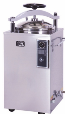
MK-35HD/MK-50HD MK-75HD/MK-100HD Vertical Pressure Steam Sterilizer Digital Display Automation Chamber volume: 35L Φ 318x450mm(MK-35HD) 50L Φ 340x550mm(MK-50HD) 75L Φ 400x600mm(MK-75HD) 100L Φ 440x650mm(MK-100HD)
