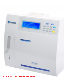
MK-AC9801 7 Parameters Semi Auto Electrolyte Analyzer Measuring Method: ISE method Sample Size: 100 \mu l Measuring Item: K, Na, Cl, Ca, pH, Calculating Item: nCa, TCa Measuring Time: 25s
