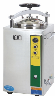
MK-35HJ/MK-50HJ MK-75HJ/MK-100HJ Vertical Pressure Steam Sterilizer Hand Round Automatic Chamber volume: 35L Φ 318x450mm(MK-35HJ) 50L Φ 340x550mm(MK-50HJ) 75L Φ 400x600mm(MK-75HJ) 100L Φ 440x650mm(MK-100HJ)
