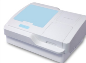
MK-DR200BN Microplate Reader Input: DIATEK ELISA Reader software Microplate types: 96/ 48 -well plate Photodetector: Silicon Photodiode Light source: 8v/50w Wavelength range: 400nm~800nm
