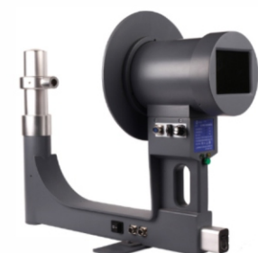
MK-IJ2 Protoble X-ray Fluoroscopy Instrument Output Image Size:Diameter 50-100mm Maxi Objective Thickness: ≤300mm Resolution: 50LP/cm
