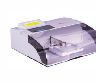
MK-SK2000A Microplate Washer Interchangeable manifolds for 8- and 12-well strips Minimal residual volume (<1µL/well) Dispense precision Cv<2% Detachable ELISA Plate pallet, convenient for the pallet clearing and sterilization
