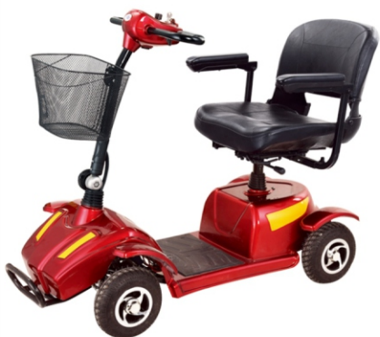
MK1-160 Foldable Mini Travel Mobility Scooter Rotary Seat, Adjustable Armrest, Easy Operating High Power Motor, High Power Controller, High Capacity Battery Distancerange: 15 KM/ONE Fully Charge
