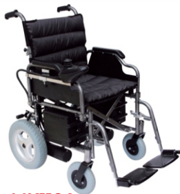
MK110A Electric wheelchair Powder Coated Steel Folding Frame Flip Up Armrest, Detachable Footrest Drop Back Handle
