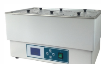
MK-HH-S6 Digital Display Thermostatic Water Bath Temperature Range: RT-100°C Temperature Homogeneity: ±1.5°C Temperature Fluctuation: ±1.5°C Working Size: 460x300x120mm
