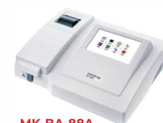
MK-BA-88A Semi Auto Biochemistry Analyzer 7.0" TFT touch-screen & pop-up keypad Two test mode: flowcell or cuvette External keyboard or mouse support via USB Built-in thermal printer Endpoint, Fixed-time, Kinetics and Absorbance Wavelengths range 340 to 670nm Up to 200 tests can be programmed
