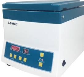
MK-LC04C Low Speed Centrifuge Speed Range: start up~4000rpm Capacity: 20mlx12 Maximum RCF: 2325xg Timing Range: 0~99mins
