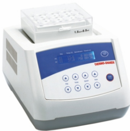
MK-200P Thermo Shaker For Micro Tubes Temperature Range: RT+5℃~100℃ Shaking Speed: 100-1200rpm Timing Range: 0-99 h 59 min
