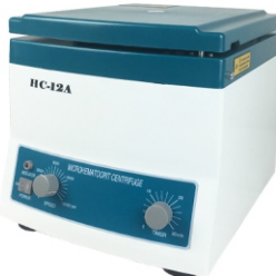
MK-HC12A Hematocrit Centrifuge Speed Range: start up~12000rpm Capacity: Φ1.5x75mmx24 capillary tubes Maximum RCF: 15300xg Timing Range: 0~30mins
