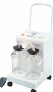
MK-7A-23D Electric Suction Apparatus Max vacuum: ≥0.08Mpa(600mmHg) Vacuum range: 0.02Mpa(150mmHg) Flow rate: ≥20L/min Suction bottle: 2500ml x 2(glass)
