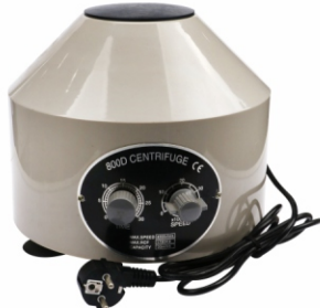
MK-800D Low Speed Centrifuge Speed Range: start up~4000rpm Capacity: 20mlx6 Maximum RCF: 1790xg Timing Range: 0~30mins
