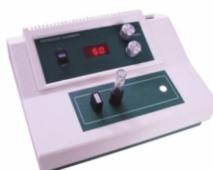
MK-AE-11D Photoelectrimeter Colorimeter Filter Glass: 420, 470, 530, 620, 660nm Or 405, 492, 546, 578, 660nm Test Tube: 10mm inner dia Light Source Tungsten Bulb: 6V 0.5A
