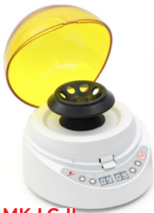
MK-LC-II Mini Centrifuge Speed Range: 3000~10000rpm Capacity: 8x0.2ml/8x0.5ml/8x1.5ml/8x2ml Maximum RCF: 5460xg Timing Range: 1s~99min
