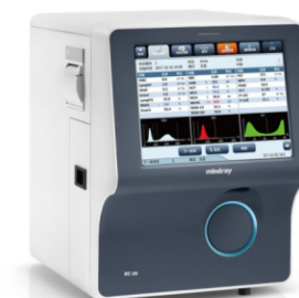
MK-BC-30 3-Diff Auto Hematology analyzer CBC+3-DIFF, 21 parameters+3histograms Throughput: 70 samples per hour 10.4 inch TFT touch screen Open vial sampling 400,000 results storage with histograms
