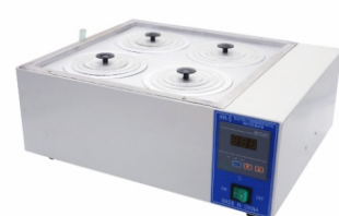
MK-HH-S Digital Display Thermostatic Water Bath Temperature Range: RT-100°C Temperature Homogeneity: ±1°C Temperature Fluctuation: ±1°C Working Size: 320x320x120mm
