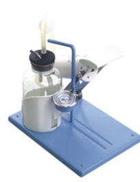
MK-7B Pedal Suction Apparatus Max vacuum: ≥0.08Mpa(600mmHg) Vacuum range: 0.02Mpa(150mmHg) Flow rate: ≥10L/min Suction bottle: 1000ml(glass)
